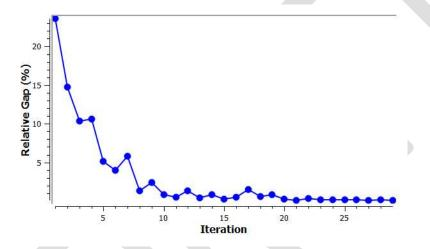
Figure 12 - AM Peak Static Assignment Convergence
