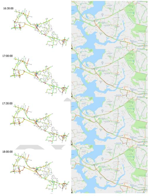
Figure 31 - PM Modelled Congestion versus Observed
