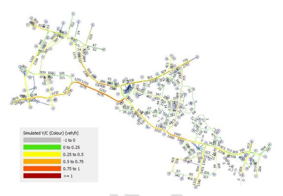
Figure 14 - AM Peak Assigned Flow in PCU/hr (6.15 am - 9.30 am)
