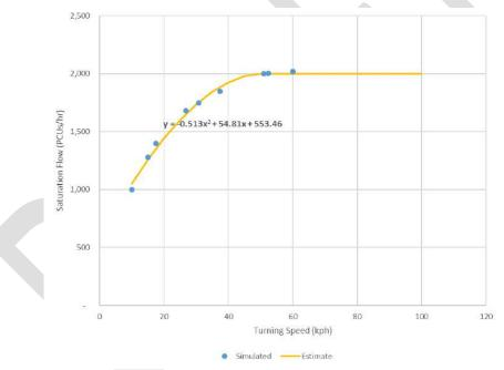
Figure 11 - Adopted Relationship between Signal Saturation Flow and Turning Speed. The line of best fit through the simulated saturation flows for turning speeds between 10 and 50 km/hr, where 10 km/hr is the minimum turning speed applied in ADTA. The saturation flow was capped at 2,000 pcu/hr/lane for turning speeds higher than 50 km/hr.
