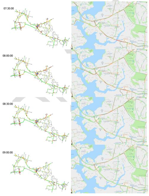
Figure 30 – AM Modelled Congestion versus Observed
