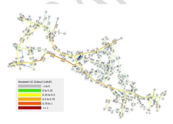
Figure 15 - PM Peak Assigned Flow in PCU/hr (3.15 pm - 6.30 pm)
